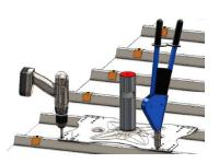
Fastening with 12 rivets or 16 self-drilling screws
